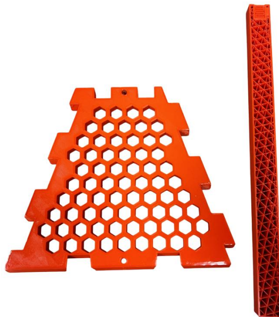
Figure 2: Individual modules designed based on light structures such as truss or honeycomb, aimed to minimize the consumption of the 3D-printing material often harmful to the environment.
