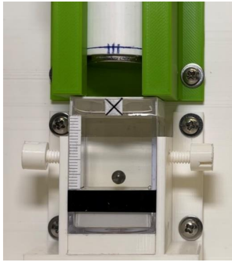
Figure 5: Successful levitation of a small magnetic bead by the setup developed in this project. The graph on the right-hand side illustrates the position x(t) of the magnetic bead versus time during the levitation process, starting at t = 0 . As shown in this graph, the magnetic bead is initially at x(0) \approx 3 mm (i.e., 3 mm below its equilibrium point), and within about 10 seconds, it reaches the steady state with an error of \pm 0.08 mm from the equilibrium.
