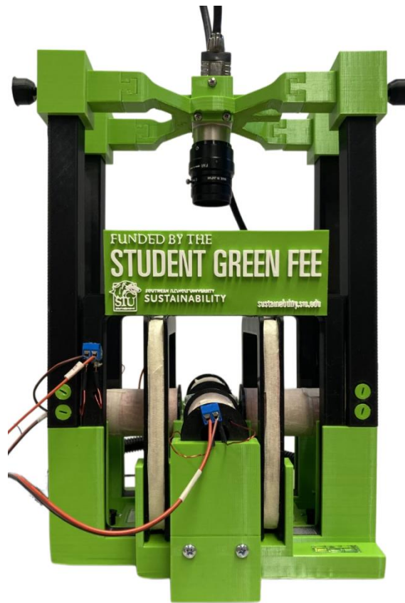
Figure 7: Magnetic manipulator, designed, prototyped, tested, and calibrated in this project. The Green Fund Marker has been 3D-printed on the fixture of the setup.
